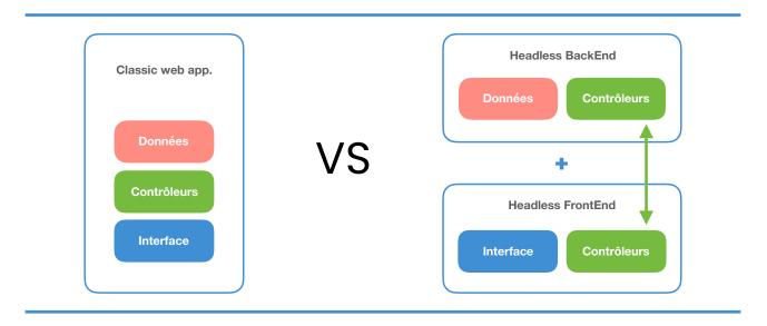
Modularity and easy maintenance The Headless architecture allows a great modularity of the software bricks for next evolutions and facilitates maintenance. This is a solution called "scalable".
